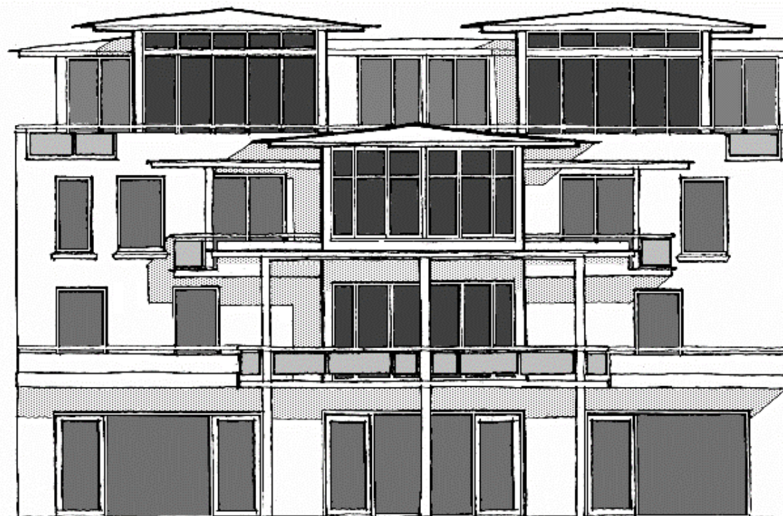
Figure 4.3.5: Street elevation illustrating desired character of buildings Note: Any fifth storey or greater should be divided into pavilion structures that are separated by terraces or roofs
