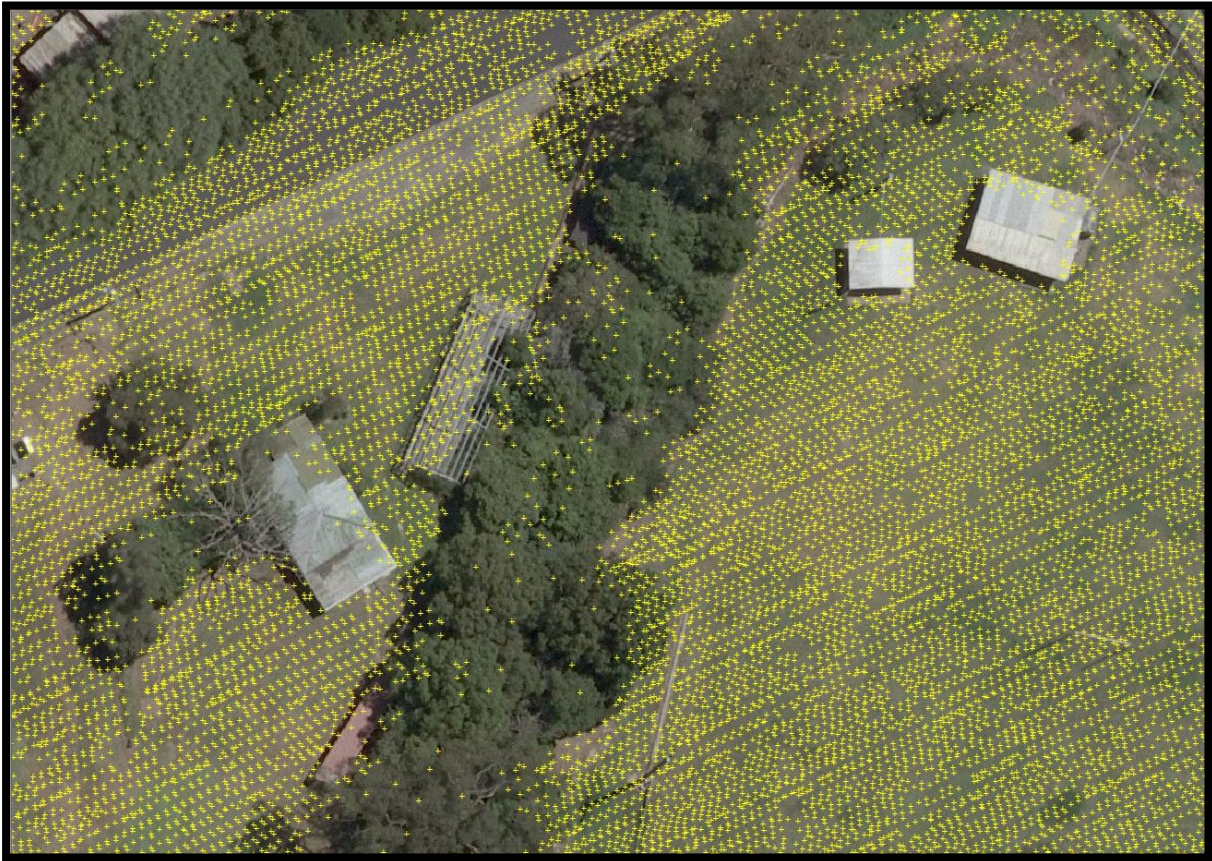
Plate 1 LiDAR data points along Chittaway Creek immediately upstream Chittaway Road showing reduced point density in areas of high vegetation density
