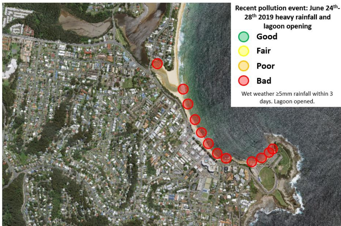
Figure 10: Water quality after large rainfall event and lagoon opening (Enterococci sampling from 24 June - 28 June 2019).
