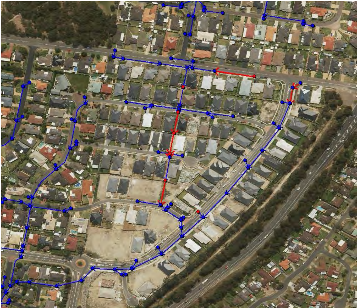
Plate 2 Stormwater Pits and Pipes that Were Updated based Upon WAE Survey (red)
