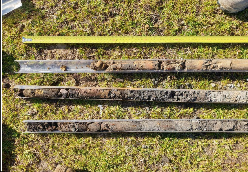
PHOTO 56: 110 PACIFIC HWY – SHOWING NATURAL SOILS DURING THE EXCAVATION OF BH067, PHOTO TAKEN 15/08/19
