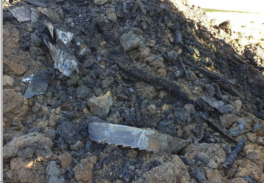
PHOTO 52: 90 PACIFIC HWY – SHOWING TP007 WHICH EXCAVATED AN AREA OF THICK FILL FOUND TO BE TYPICAL OF THE EAST / SOUTH OF THE LOT, PHOTO TAKEN 13/08/19
