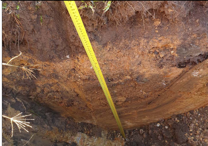
PHOTO 59: 110 PACIFIC HWY – SHOWS A TEST PIT (TP071) WHICH GIVES A TYPICAL EXCAVATION PROFILE FROM SURFACE IN THE NORTHERN LOTS, PHOTO TAKEN 15/08/19
