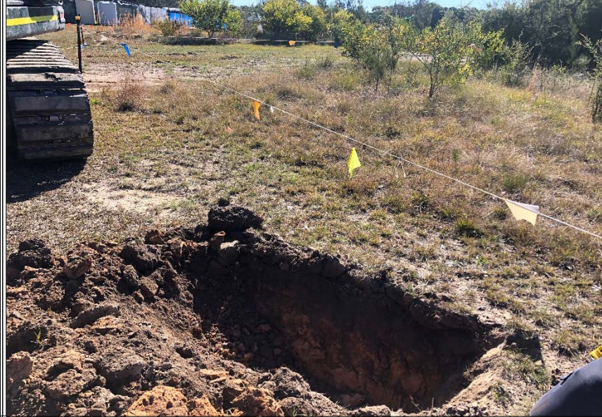
PHOTO 60: 110 PACIFIC HWY – SHOWING AN EXAMPLE OF THE DOMINANT NATURAL MATERIAL FROM TP116, THAT WAS FOUND UNDERLYING THE MAJORITY OF SITE, PHOTO TAKEN 15/08/19
