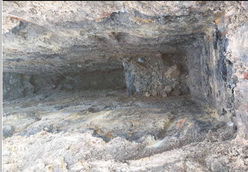
PHOTO 52: 90 PACIFIC HWY – SHOWING TP007 WHICH EXCAVATED AN AREA OF THICK FILL FOUND TO BE TYPICAL OF THE EAST / SOUTH OF THE LOT, PHOTO TAKEN 13/08/19
