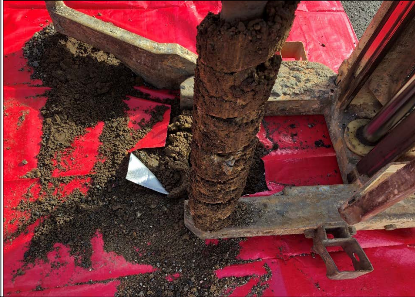
PHOTO 20: 49-65 WENTWORTH AVE – SHOWING MATERIAL RECOVERED FROM BH002/MW02 FROM 2.0M-2.5M DEPTHS, PHOTO TAKEN 12/08/2019
