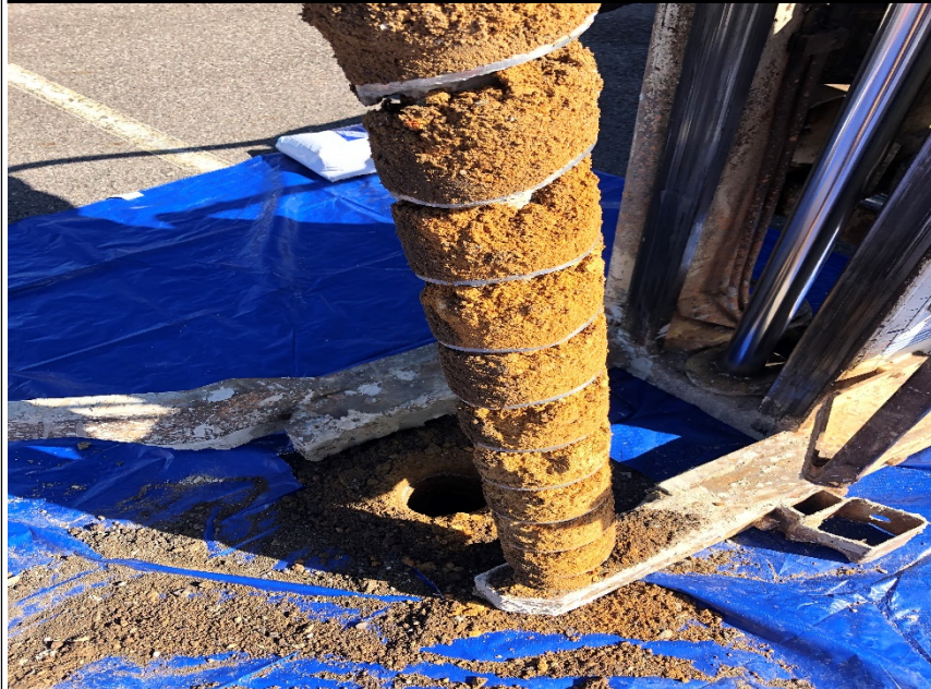
PHOTO 20: 49-65 WENTWORTH AVE – SHOWING MATERIAL RECOVERED FROM BH002/MW02 FROM 2.0M-2.5M DEPTHS, PHOTO TAKEN 12/08/2019
