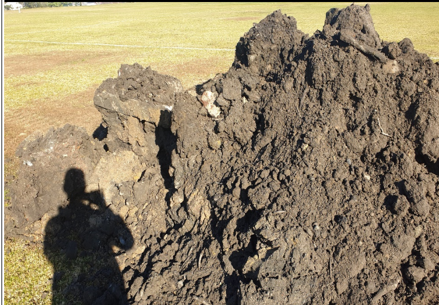
PHOTO 14: 90 PACIFIC HWY – TP36 THICK FILL FOUND TO BE TYPICAL OF THE EASTERN PORTION OF SPORTS FIELD, 13/08/19
