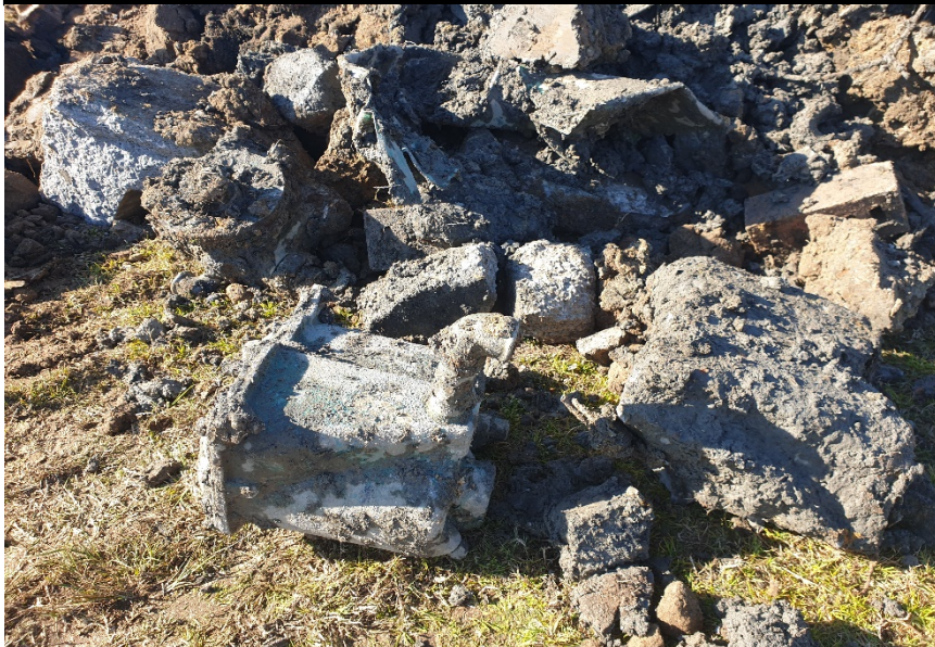
PHOTO 13: FILL FROM TP008 IN THE SOUTHERN PORTION OF SPORTS FIELD, WHICH INCLUDED A LARGE VOLUME OF DEMO WASTE AND ENGINE PARTS, 13/08/19
