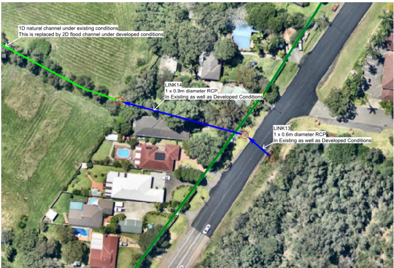
Figure 5-7 Location of Conduits in the vicinity of the Central Coast Highway
